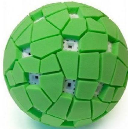
The panoramic camera solves all these problems. The camera is thrown into air and captures the image at the highest point of flight (when it is hardly moving). The camera takes full spherical panoramas, requires no preparation and images are taken instantaneously.
