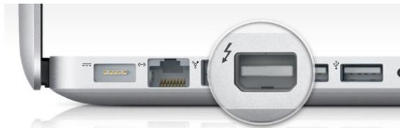
Thunderbolt combines PCI Express and Display Port into a serial data interface that can be carried over longer and less costly cables. A single Thunderbolt port supports hubs as well as a daisy chain of up to seven Thunderbolt devices; up to two of these devices may be high-resolution displays using Display Port. Existing Mini Display Port adapters for DVI, dual-link DVI, HDMI, and VGA are compatible with Thunderbolt.
