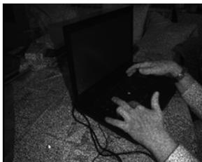
This infrared image shows the laser grid, that Kinect uses to calculate depth.
