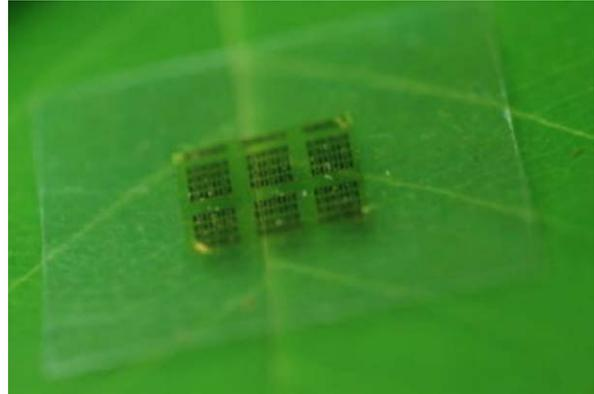
with the capacity for thermal expansion, they found that CNF worked the best over the petroleum-based polymers. The team's next challenge is to show that even a wood-based chip could perform just as well as existing gallium arsenide-based microwave chips.
