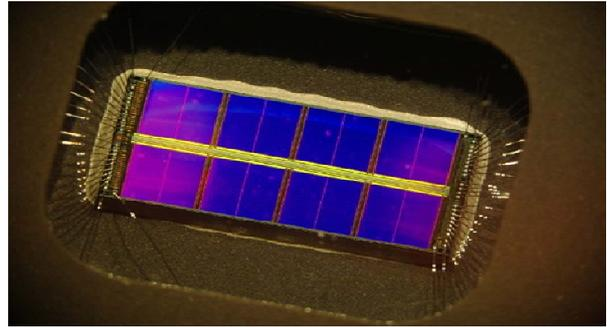
This team has now managed to find a way to modify a type of glass known as chalcogenide - which is already used in optical devices such as CDs and DVDs - so that they can be used alongside the current systems. Chalcogenides have some useful properties like they're able to conduct light across a pretty wide range of bandwidths.
