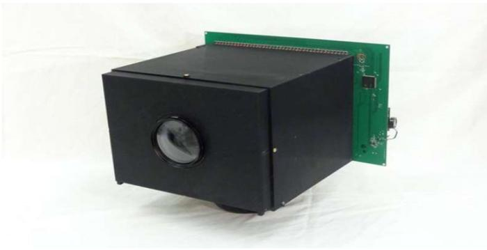
A Professor of Computer Science at Columbia Engineering, has invented a prototype video camera that is the first to be fully self-powered. It can produce an image each second. They designed a pixel that can not only measure incident light but also convert the incident light into electric power.
