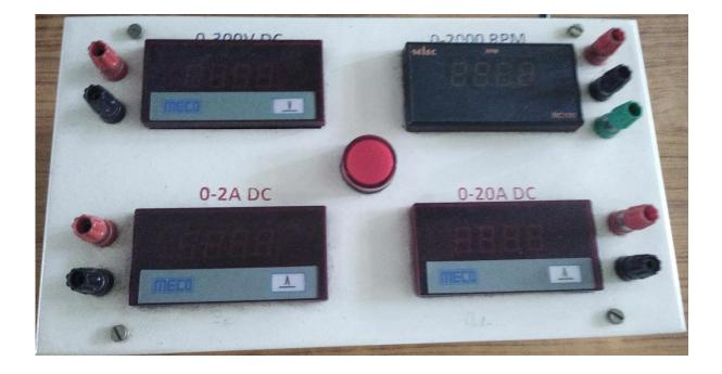
This box is used for measuring D.C Voltage, DC current and speed of DC motor.
