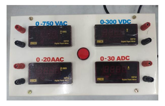
This is useful for measuring AC Voltage DC Voltage AC Current and DC Current.
