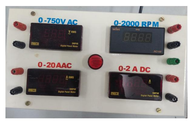
This box is used for measuring AC voltage, AC current and DC current and speed of alternator.
