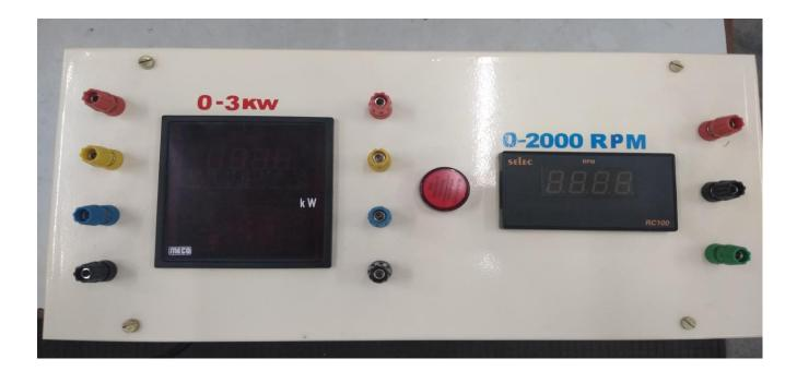
This box is used to measure power and speed of AC motor.
