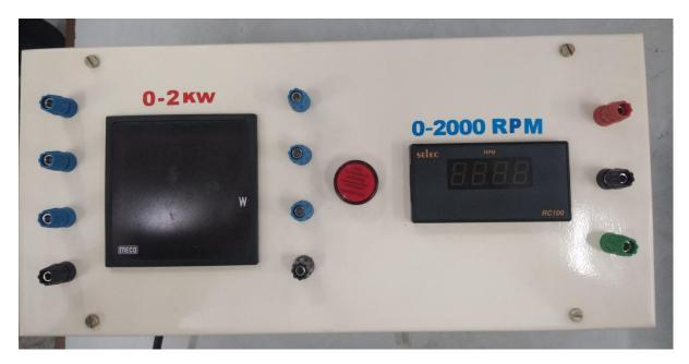
This box is used to measuring power and speed of AC motor.
