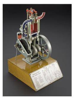
Piston, connecting rod , crank are binary links.
