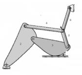
3. Quaternary joint: If four links are joined at the same connection, it is known as quaternary joint. It is equivalent to three binary joints.
