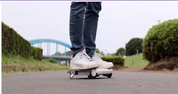
Kuniako Saito, a Japanese engineer, and his team at Cocoa Motors, have created a laptop-sized personal vehicle that weighs less than seven pounds. The device, dubbed the 'WalkCar', is described as a 'car in a bag' because it can easily be carried around. It's sort of like a small, four-wheeled electric skateboard meets a Segway. The device is powered by lithium batteries and comes in both indoor and outdoor models. It
