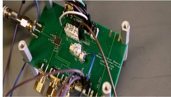
must travel in the same manner in forward and reverse directions. The researchers used a series of switches that emulate the effects of magnetism by rotating signals across a set of capacitors. This ends up negating reciprocity and enabling two-way signals on a single radio antenna.
