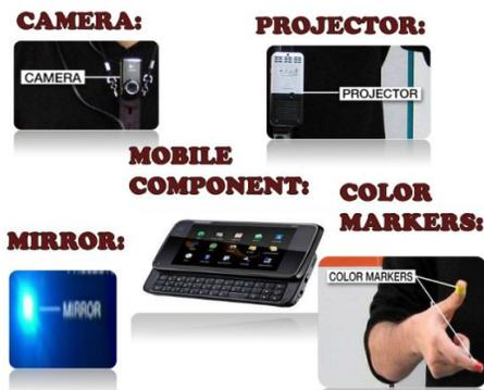
\Sixth Sense Technology is neck worn gestural interface device that builds up the physical world around us with the digital information and enables the users use natural hand gestures to connect with the such information. It is a pendent like device that consist two main components; a data projector and a camera. This technology enables the user to connect with the internet nersistentlv.
