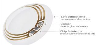
Google's smart contact prototypes squeeze a glucose sensor, antenna, capacitor and chip between two contact lens layers, making a kind of electronics sandwich. A tiny hole on the eye side allows tear film, which contains glucose, to reach the sensor. The integrated circuit is no larger than a piece of glitter, and its weight is undetectable on the tip of a finger. The sensor, which takes glucose readings twice a second, isn't much bigger. And the antenna is thinner than a human hair.
