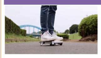
Kuniako Saito, a Japanese engineer, and his team at Cocoa Motors, have created a laptop-sized personal vehicle that weighs less than seven pounds. The device, dubbed the 'WalkCar', described as a 'car in a bag' because it can easily carried around. It's sort of like a small, four-wheeled electric skateboard meets a Segway. The device is powered by lithium batteries and comes in both indoor and outdoor models. It model, but can carry a person of upto 120 kgs.
