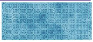
requirements for the memory to function, it may still be a while yet before your Spotify or Netflix streams to you courtesy of chlorine. In its current form the memory can operate only in very clean vacuum conditions and at liquid nitrogen temperature, so the actual storage of data on an atomic scale is still some way off. But through this achievement they have certainly come a big step closer.
