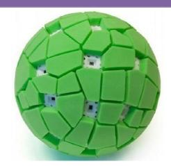
The panoramic camera solves all these problems. The camera is thrown into air and captures the image at the highest point of flight(when it is hardly moving). The camera takes full spherical panoramas, requires no preparation and images are taken instantaneously.
