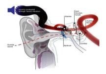
Bone conduction is the conduction of sound to the inner ear through the bones of the skull. Bone conduction allows you to hear sound through the vibration of bones of your face (jaw bones and cheek bones). These devices decode sound waves and convert them into vibrations that can be received directly by the cochlea so that ear drum is never involved. In this Premiumpitch technology is used. With bone conduction you are free to enjoy your music while keeping your ears open to
