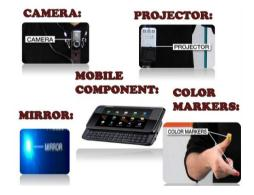
\Sixth Sense Technology is neck worn gestural interface device that builds up the physical world around us with the digital information and enables the users use natural hand gestures to connect with the such information. It is a pendent like device that consist two main components; a data projector and a camera. This technology enables the user to connect with the internet persistently.
