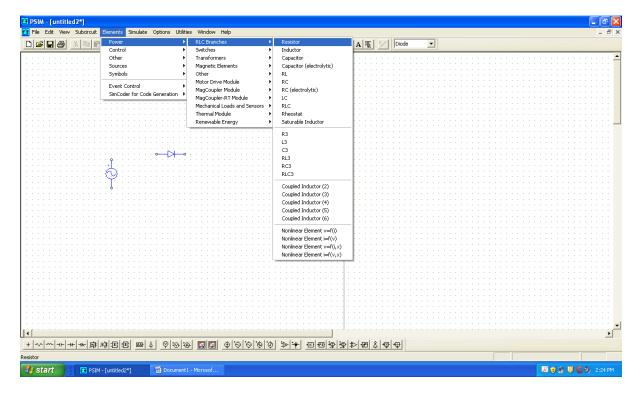
Hint: To rotate the element click right button of the mouse after selecting the element.
