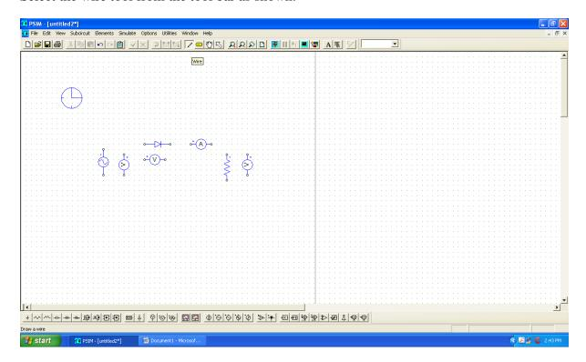
Connect the elements using the wire tool selected from the tool bar.
